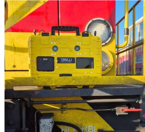
SAMIRAmobil w/ RADAR, LiDAR, Stereo camera, GNSS and 5G data transmission
