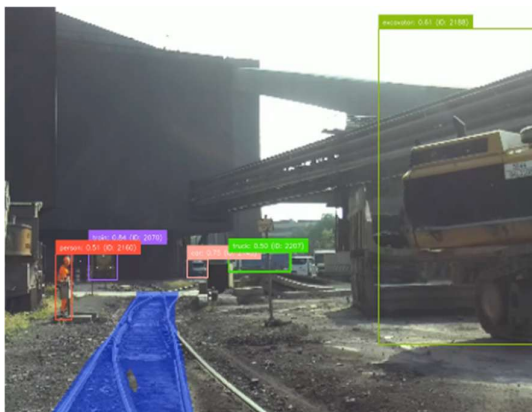
Augmented video stream displayed to the driver
